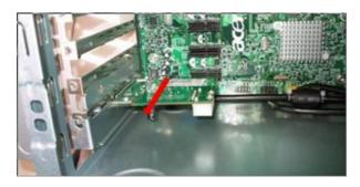
3.6 Pull the leaver outwards a little to release the PCI latch then remove other add-on card.
